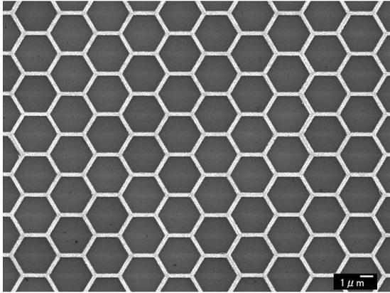
Fig. 1: SEM image of a honeycomb network with about 2500 cells, lattice constant of  $2 \mu\text{m}$  and line width of  $0.2 \mu\text{m}$ .
