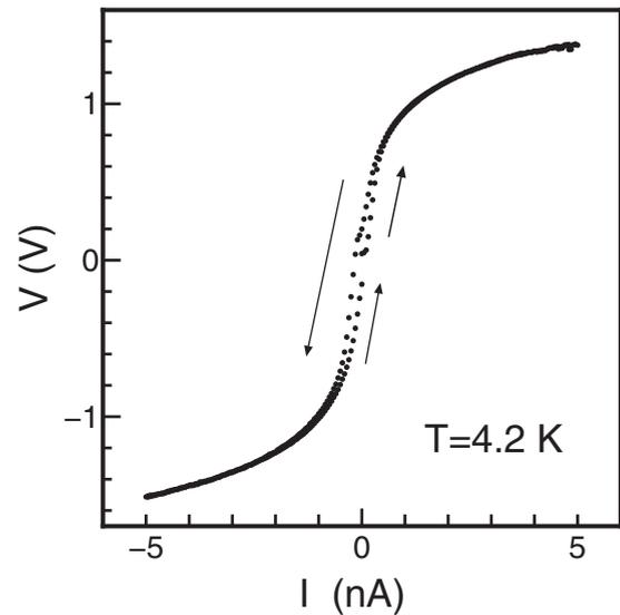
FIG. 2. Current-voltage ( $I$ - $V$ ) characteristics of the  $o$ -TaS<sub>3</sub> sample observed at 4.2 K. The  $I$ - $V$  curve is significantly nonlinear. A slight hysteresis is found near  $I = 0$  as shown by the arrows.
