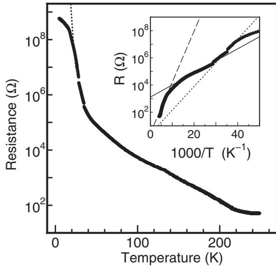
FIG. 1. Temperature dependence of  $o$ -TaS<sub>3</sub>. The discontinuity is caused by a change in the measurement current. Inset shows three Arrhenius fits for high, intermediate, and low temperature ranges, denoted by broken, solid, and dotted lines, respectively. The low temperature fit is also shown in the main panel by the dotted line, by which the extrapolation of the ohmic resistance at 4.2 K appears to exceed  $10^9 \Omega$ .
