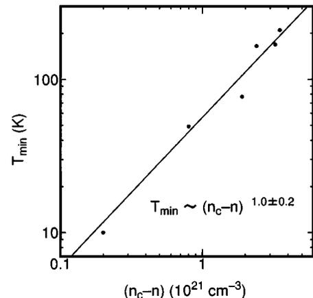
FIG. 4. Relation between the resistivity-minimum temperature  $T_{\min}$  and the carrier concentration  $n$ .
