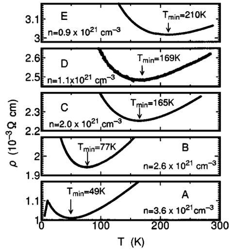
FIG. 3. Resistivity minima of samples A, B, C, D, and E. The temperatures of the resistivity minima depend on the carrier concentration.
