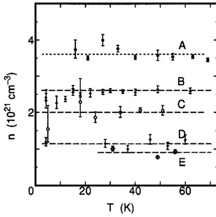
FIG. 2. Carrier concentration of samples A, B, C, D, and E, determined as  $n=1/R_H e$ , where  $R_H$  is the Hall coefficient. The carrier concentration becomes smaller when a significant amount of Sr is substituted by Bi. It is shown that the Hall coefficient of each sample is independent of temperature.
