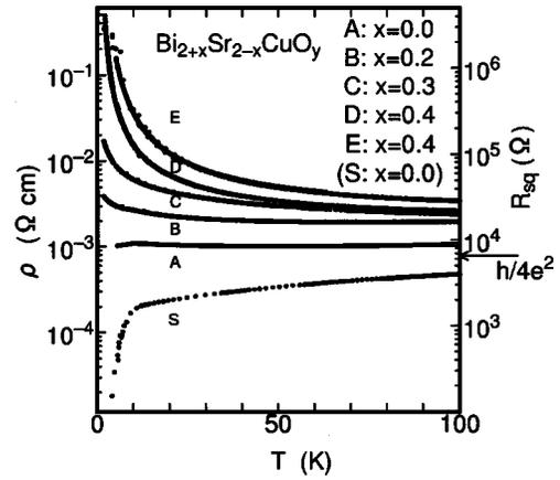
FIG. 1. Resistivities of the samples with different Bi/Sr ratio. The sheet resistance of 1 k $\Omega$  corresponds to the resistivity  $1.2 \times 10^{-4} \Omega \text{ cm}$ . The residual resistivity becomes higher when a significant amount of Sr is substituted by Bi.
