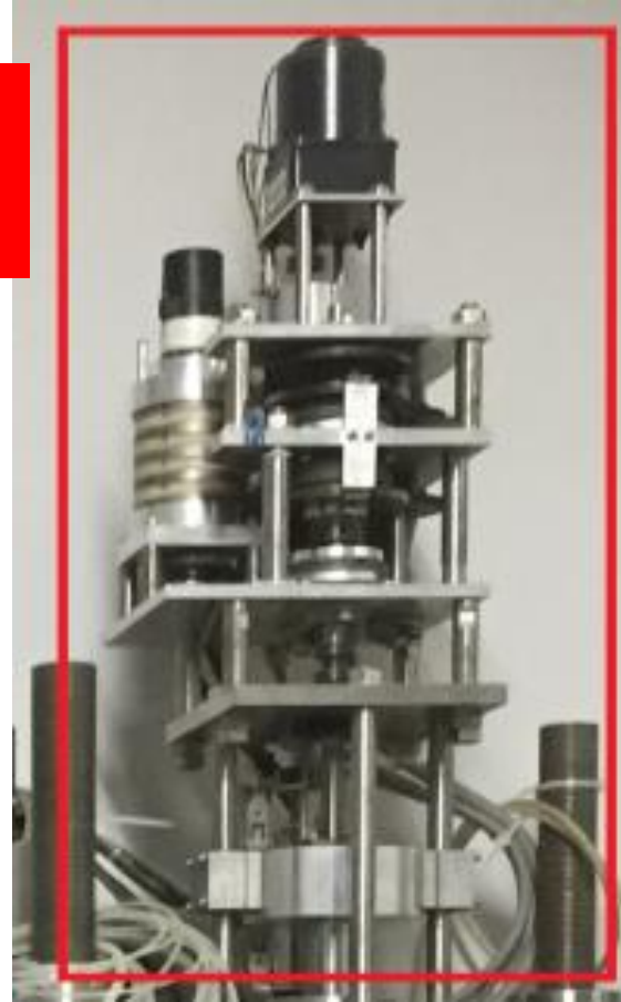
Motor-driven loading device (Zhao, 2018)
