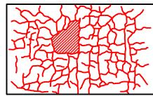
漏水が顕著となり、押抜き せん断破壊が発生 After the increase of the water leakage, punching shear failure occurs.
