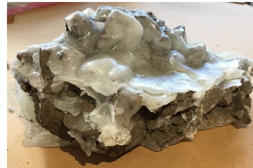
Ballast sample by Wax-coating method
