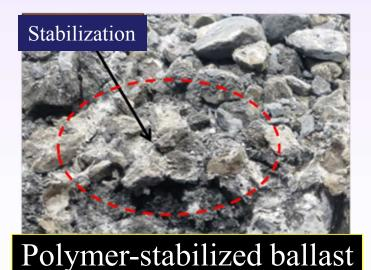
• PVA reacts with sodium silicate to form gel thereby it is possible to perform the stabilization of the fouled ballast.
