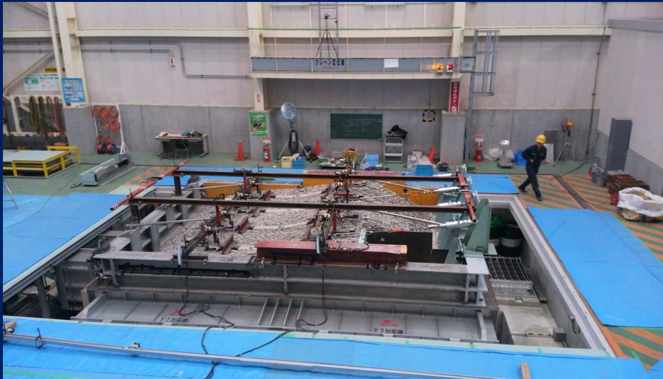
Shaking table tests on a full-scale ballasted track (Nakamura et al. 2014)
