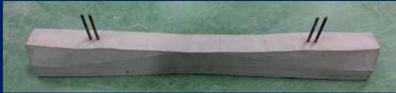
3H sleeper (in 1/5th scale) Ballast settlement S = 0, 10, 20, 30\text{mm}
