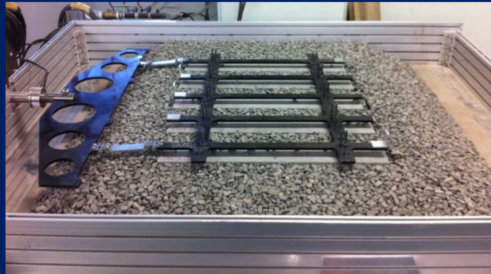
Track panel pull-out test on 1/5-scale models (Koike et al. 2014)
