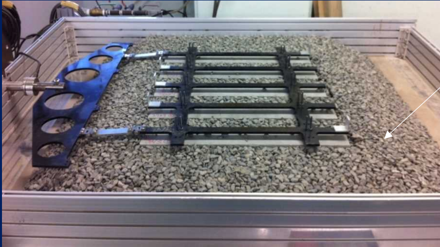
1/5th scale model for track panel pull-out test
