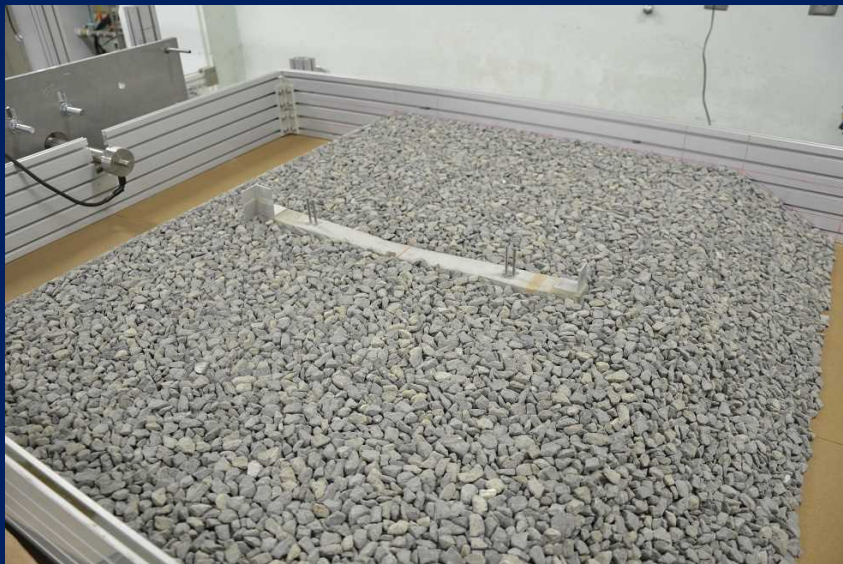
Single-sleeper pullout tests
