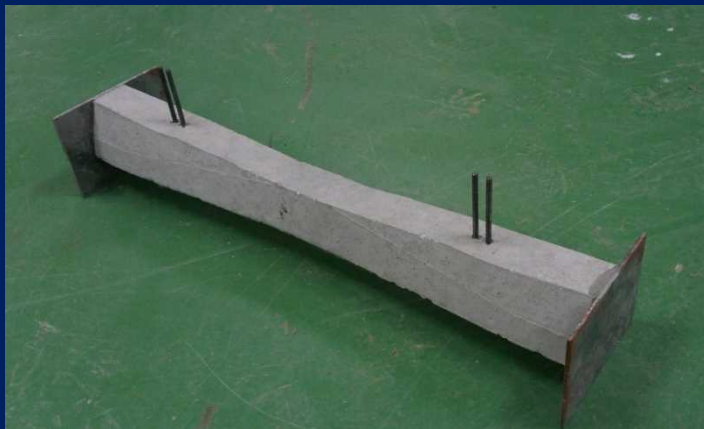
3H sleeper with buckling prevention plates (in 1/5th scale) Ballast settlement S = 0, 10, 20, 30, 40\text{mm}
