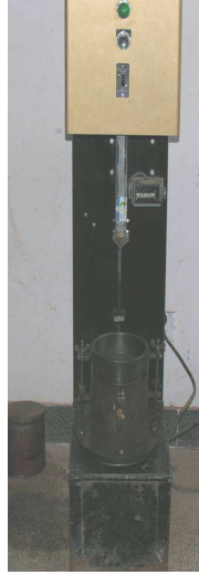
击实仪及击实制样 Compaction test apparatus and compaction sample preparation
