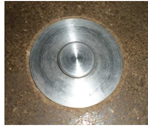
传力架底面与击入土体的承载板 Bottom of force transmit frame and load plate buried into the soil
