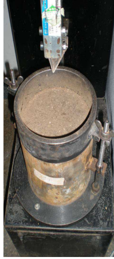
击实仪及击实制样 Compaction test apparatus and compaction sample preparation
