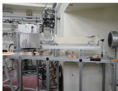
Fig.1 Intermediate-angle neutron scattering instrument iANS.
