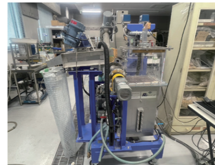
図1 ジグ選別機です。右側に見える透明な水槽内で選別を行います。 Figure 1 : This is JIG separation machine. The separation is treated in the water tank at the right side.
