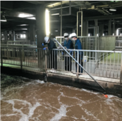
図2 下水処理施設における活性汚泥の採取 Figure 2 : Activated sludge sampling at an waste water treatment plant.
