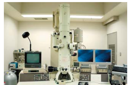
図2 材料の微細構造解析に有効な透過型電子顕微鏡 Figure 2: Transmission Electron Microscope used for microstructural analysis of materials.
