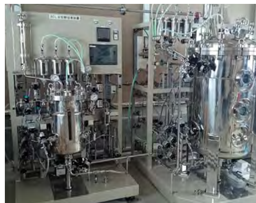
図1 大型発酵培養槽 Figure 1: A large sized fermentor.
