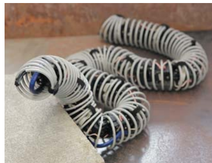
図1 車輪を持たず地面を這って進むヘビ型ロボット Figure 1: A snake robot without wheels; crawling on the ground
