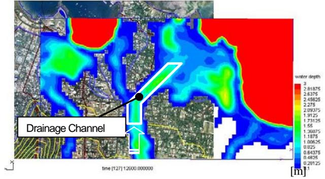
Fig.8. Water Depth at the Maximum Discharge with Drainage Channel (Compared with Fig.5.)
