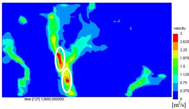
Fig.7. Velocity Contour at Maximum Discharge
