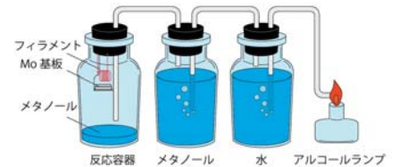
図1 君にも作れるダイヤモンド合成装置 Figure 1: A diamond growth system for you.
