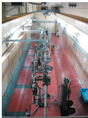
図1 工学部の45MeV電子線形加速器 Figure 1 : 45MeV electron linac at School of Engineering, Hokkaido University.
