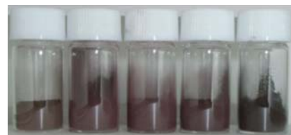
図1 粒径の異なる銅ナノ粒子材料 Figure 1 : Copper nanoparticles with various sizes
