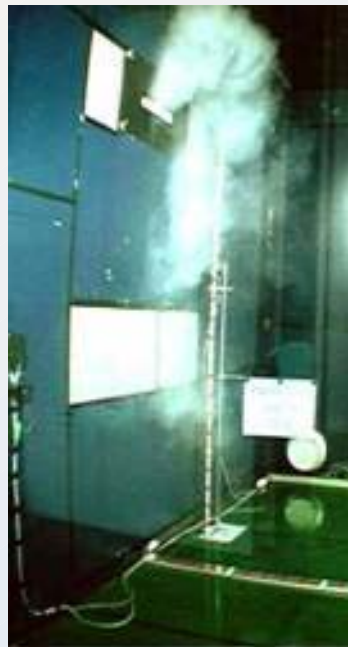
• Air flow visualization and comfort measurements in the room climate laboratory
