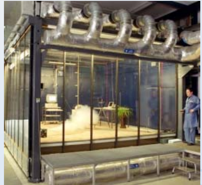
• Air flow visualization and comfort measurements in the room climate laboratory
