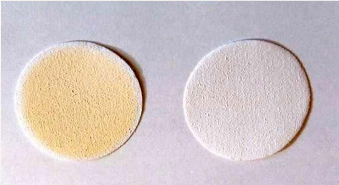
Filter for non volatile substances
