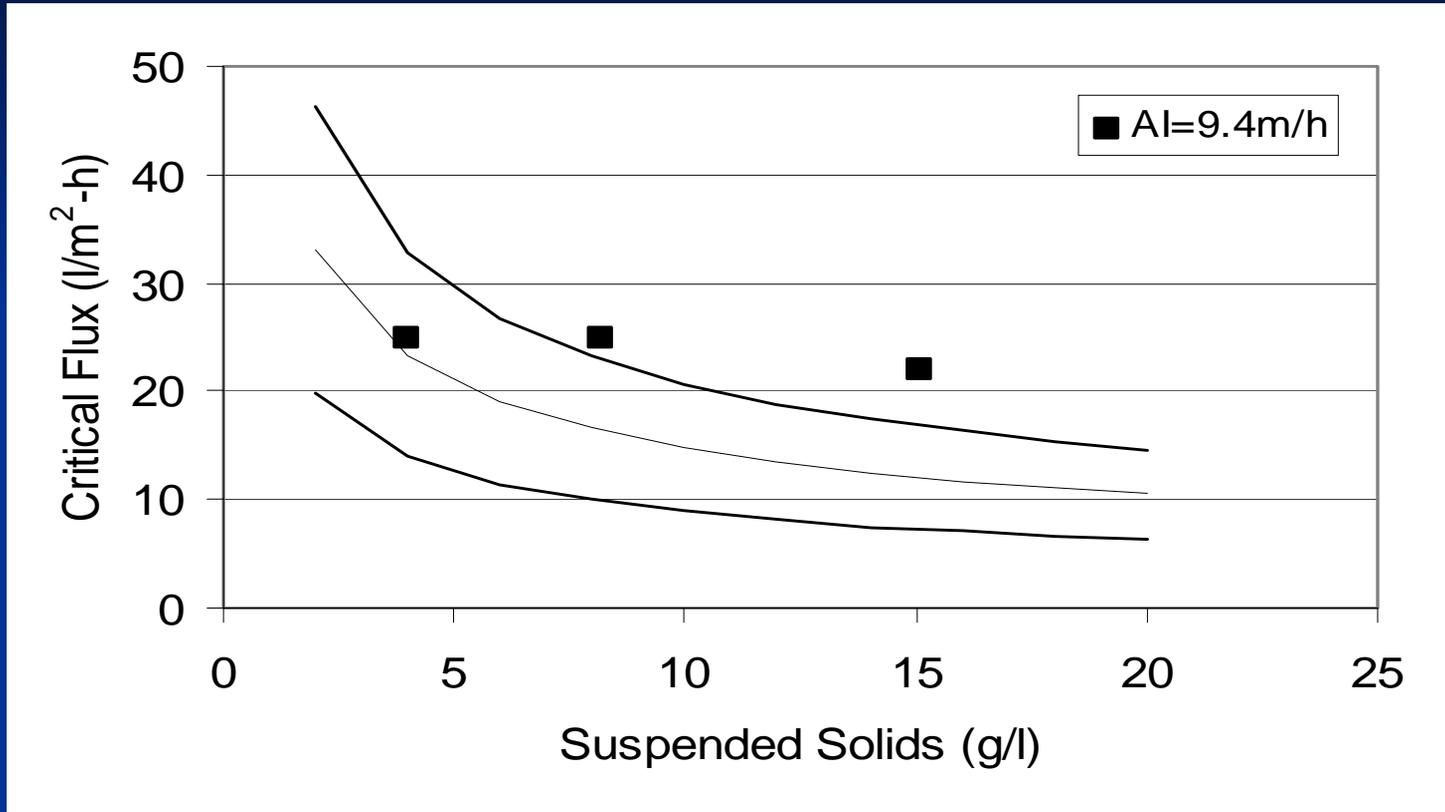
Effect of suspended solids concentration on critical flux at IMBR cross flow velocities between 0.3, 0.5, and 0.7 m/s (solid lines from Shimizu et al. (1996b) using  $K = 2.6 \cdot 10^{-5} \text{ kg}^{0.5} \text{ m}^{-1.5}$ , and  $\phi = 1$  for  $J_{ss} = K \cdot u^* \phi \cdot C_b^{-0.5}$ ), and AI=9.4 m/h (symbols for Bouhabla et al., 1998). Similarly to the EMBR results, the IMBR result of Shimizu et al. (1996b) shows a zone of rapid flux decline, followed by a zone of stabilized flux.
