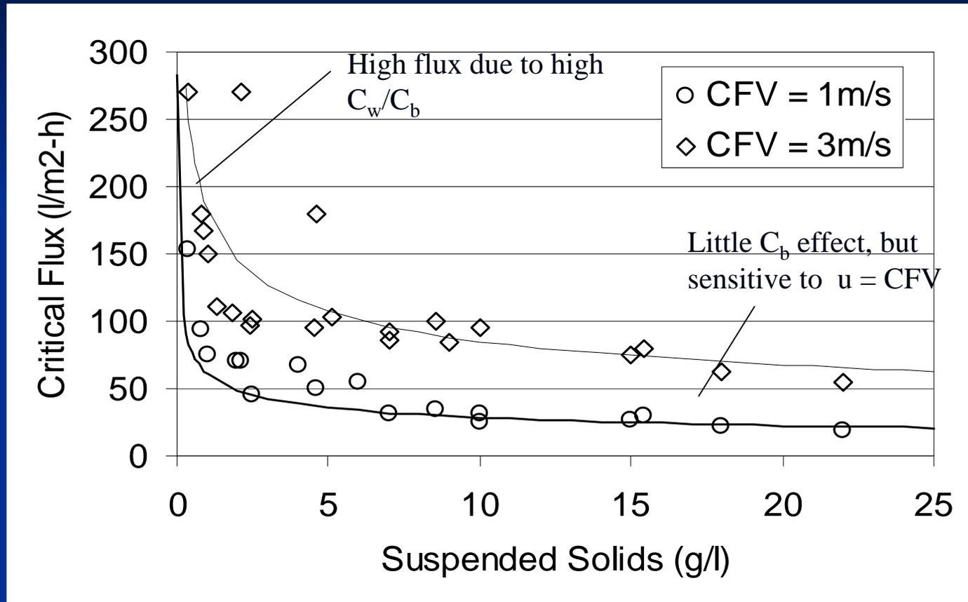
The shear-induced diffusion model (Eqn. 1) using the friction factor expression for laminar flow gives a good fit to all the data when  $a = 1.5 \mu\text{m}$ .
