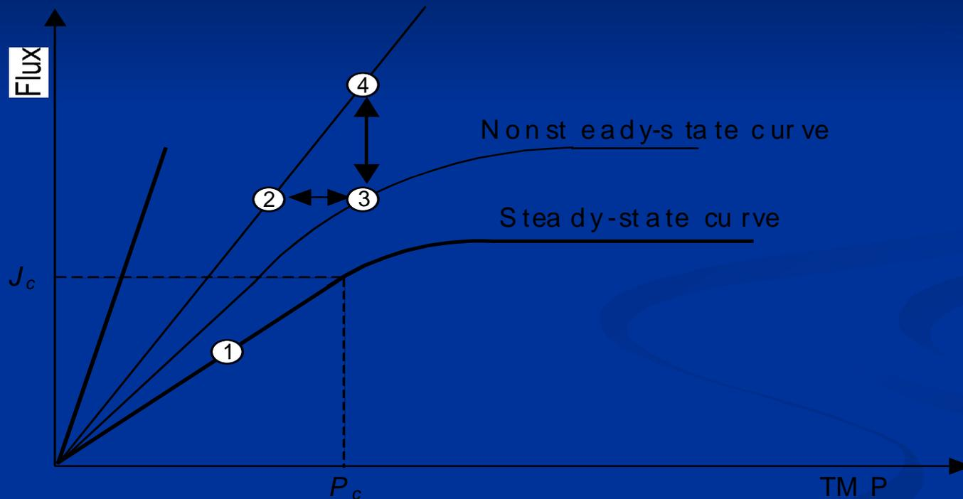
Sub-critical operation (point 1) is steady state, relying only on shear to keep  $J > J_c$  at all times. Supra-critical operation is non-steady state and requires periodic backpulsing to remove cake resistance for constant-flux operation (between points 2 and 3) or constant-TMP operation (between points 4 and 3).
