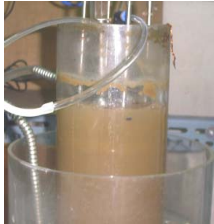
Suspended Growth Reactor (MLSS: 2,000~5,000 mg/L)
