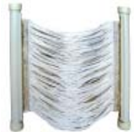
After physical membrane cleaning
