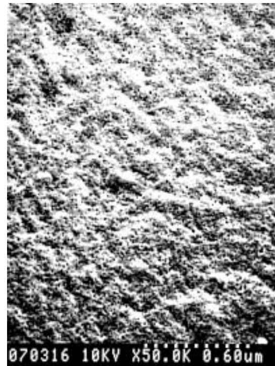
Pore size: 0.01 micrometer
