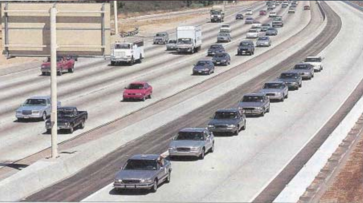
An eight-car platoon of PATH-automated Buick LaSabres on the express lane of I-15 in San Diego, Calif. "Drivers" are waving their hands out the window to demonstrate automated steering.
