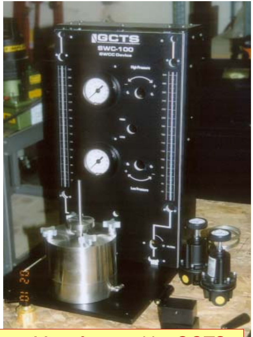
SWCC Apparatus Manufactured by GCTS
