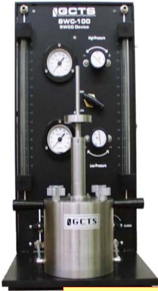
SWCC Apparatus Manufactured by GCTS
