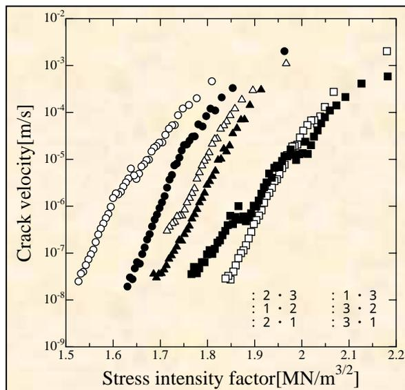
Fig. 7 Anisotropy of subcritical crack growth in Oshima granite.
