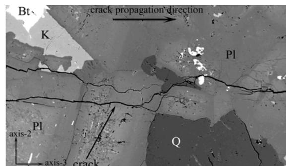
Fig. 9 Image of the crack path obtained by EPMA. (0.9 × 1.5mm)
