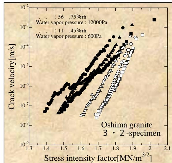
Fig. 8 Environmental dependence of subcritical crack growth in Oshima granite.
