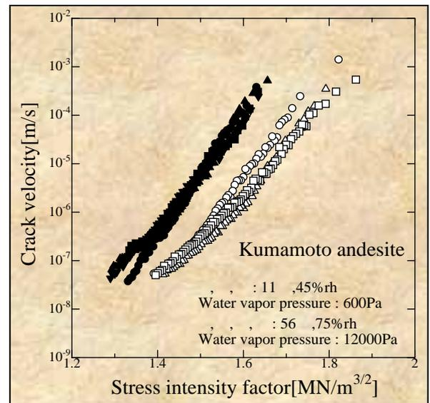
Fig. 4 Results of DT tests for Kumamoto andesite.
