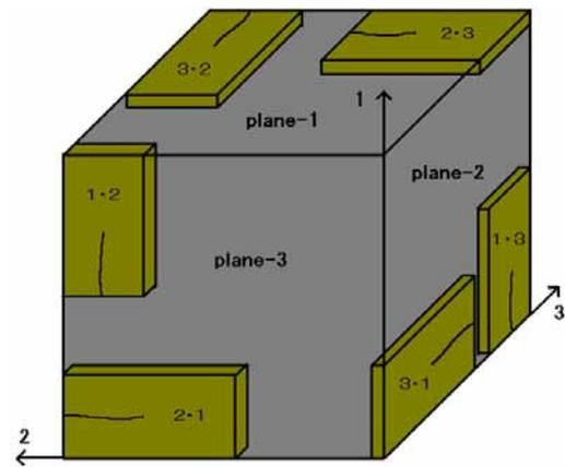
Fig. 6 Specimen preparation for granite.
